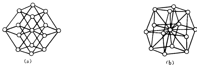
Fig. 1 Initial structure of body-centered cubic (bcc) Si_{15} (a) and its optimized result (b)
