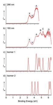
Fig. 1 Photoelectron spectra of  $TaB_{20}^-$  at 266 nm (4.661 eV) (a) and 193 nm (6.424 eV) (b) and comparison with simulated spectra of isomers 1 (c) and 2 (d) at the SAOP/TZP level.
