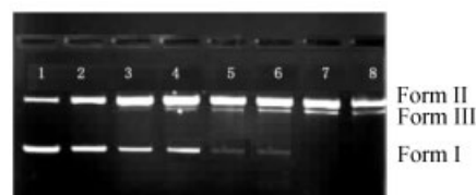
Figure 5 Agarose gel electrophoresis patterns for the cleavage of DNA by various concentrations complex. Lane 1 DNA; lane 2—8 [ c_{\text{complex}}/(\text{mol} \cdot \text{L}^{-1}) ]: 10^{-5} , 5 \times 10^{-5} , 10^{-4} , 5 \times 10^{-4} , 10^{-3} , 3 \times 10^{-3} , 5 \times 10^{-3} .
